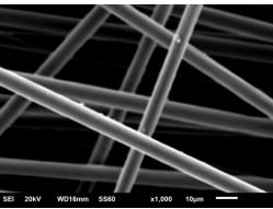
Figure1 Carbon fiber used as anode
