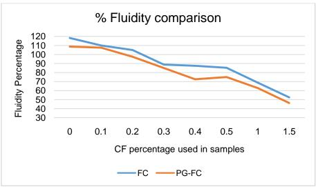
Figure 5. Fluidity % comparison between the two different types of CRM mixtures.
