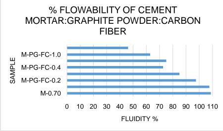
Figure 4 Fluidity percentage attained for mixtures with CF and GP
