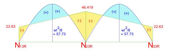
Fig. 4 B.M.D of Roof Beam 1 & 2
