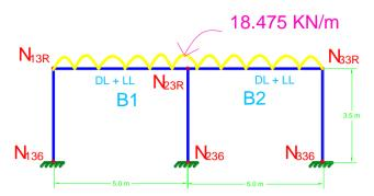
Fig. 2 Substitute Frame for Beam 1 & 2
