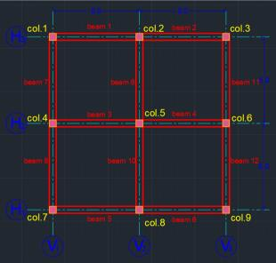
Fig. 1 Ground Floor Framing Plan
