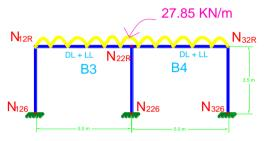
Fig. 3 Substitute Frame for Beam 3 & 4
