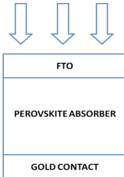
Fig.1(a). Perovskite device structure.
