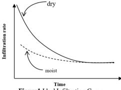
Figure1.Ideal Infiltration Curve
