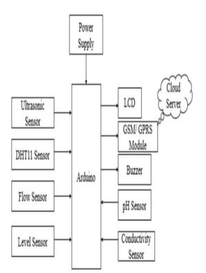
Figure 5.1: Block Diagram
