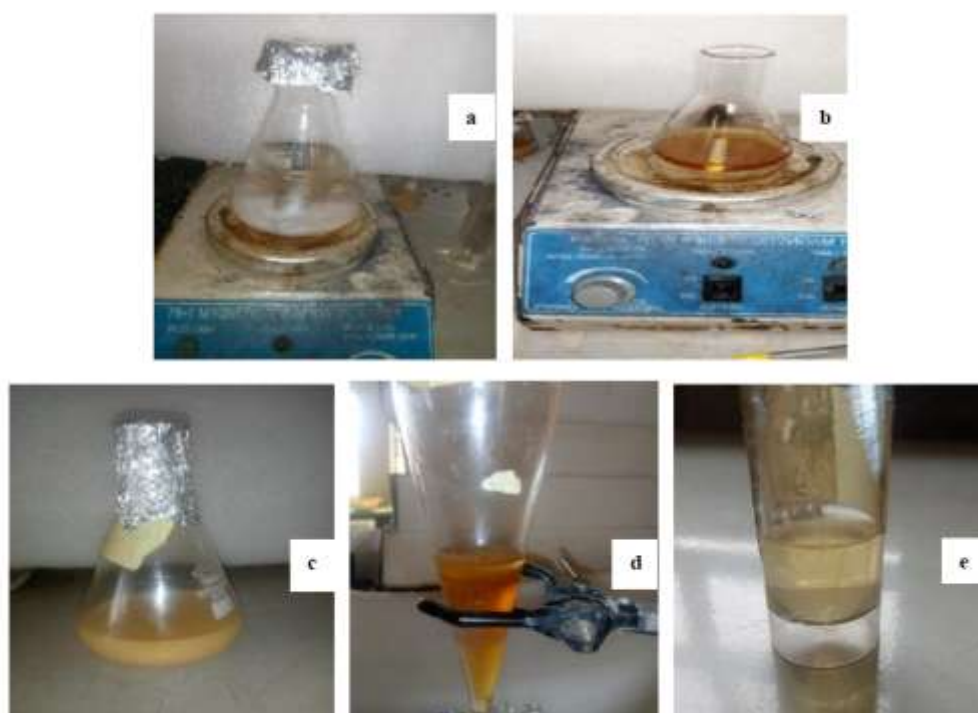
Figure 4: (a) methanol and ethanol mixture, (b) heated WCO, (c) transesterification process, (d) mixture after overnight, (e) Biodiesel after separation
