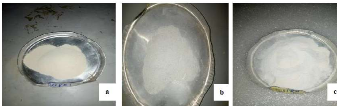
Figure 3 Calcined/pulverized eggshells (a) Turkey eggshell, (b) Duck eggshell, (c) Guinea fowl eggshell.
