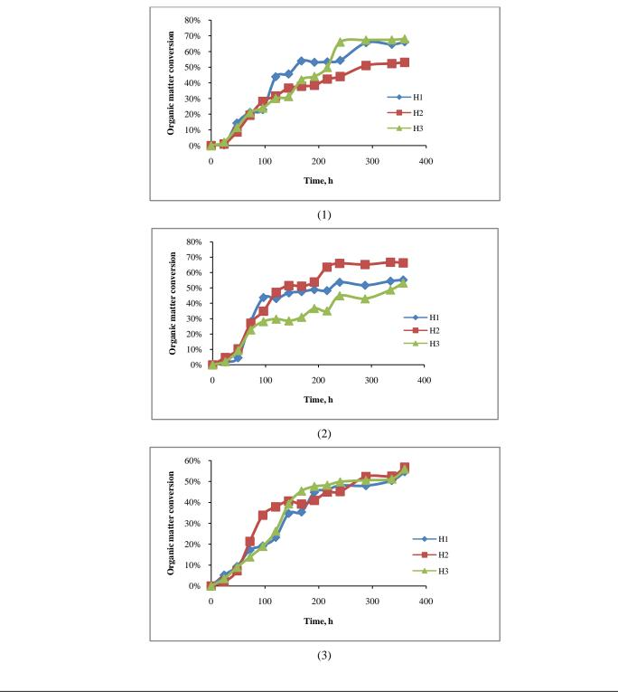
Figure 2. Organic matter conversion for the second experiment in three reactors at three differnet heights
