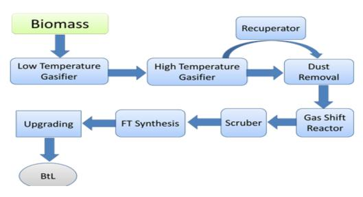
The main catalytic process to convert the syngas into a liquid fuel is known as Fischer-Tropsch (FT). This process occurs at high temperatures; it consists of a reaction between hydrogen and carbon monoxide that is explained by the following equation:
