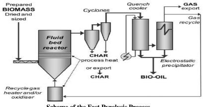
Scheme of the Fast Pyrolysis Process
