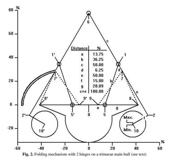
Fig. 2 shows a mechanism with 2 pivot points 5 and 5' on the main hull of a trimaran. Other points correspond to those in Fig. 1 with a few exceptions. Points on the connecting half beams (a+e) between points 6 and 2 or 2' respectively don't produce exact ellipses during folding, and no point gives an exactly horizontal
