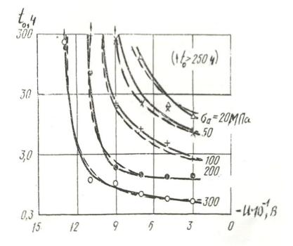
Fig.1. Dependence of the time to failure of rods made of chromium-nickel steel 18-9 in boiling solution  $MgCl_2$  on constant values of tensile stress and potentials: solid lines are the data of H.Terness experiments, broken lines are the calculations by formula (7).
