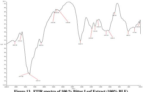
Figure 13 FTIR spectra of 100 % Bitter Leaf Extract (100% BLE)
