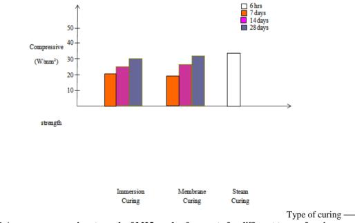
Fig-1 Average compressive strength of M25 grade of concrete for different types of curing.
