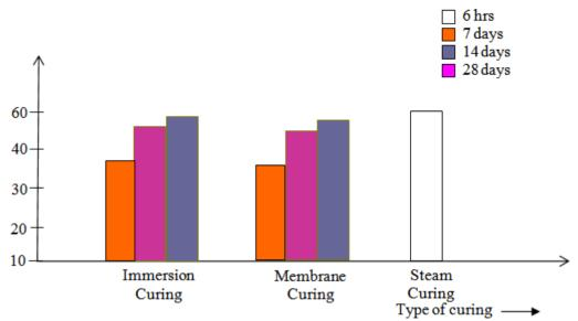
Fig-2 Average compressive strength of M30 grade of concrete for different types of curing.
